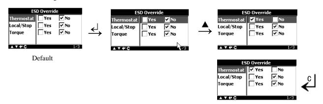
Local/remote overriding means ESD command is executed even if the selector switch does not point to remote.
