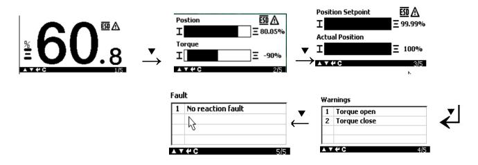
2.3.3 When the actuator is in debug state, if no any operation in 5 minutes, the screen returns to home page automatically, the home page is configurable.
